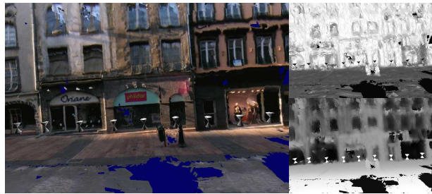
Figure 6. Three textured-mapped views of the Old Town global model (including cameras), obtained with local 3D model selection and reliability conditions. Patch orientations (or depth map) are also drawn using gray levels.
