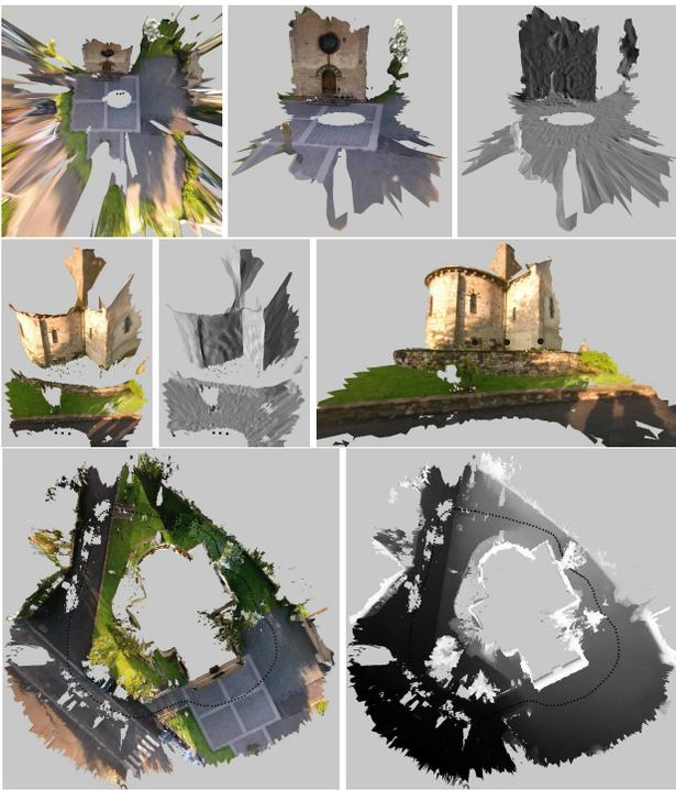
Figure 3. Several views of 3D models obtained with the catadioptric camera. Top and middle: views of two local models (3 consecutive poses) with rejection of unreliable triangles ( $R_0 = 0.08$ ), except at the top left corner. Triangle orientations are also drawn using gray levels. Bottom: top view and height map of the global model (208 poses) with rejection ( $R_0 = 0.05$ ).
