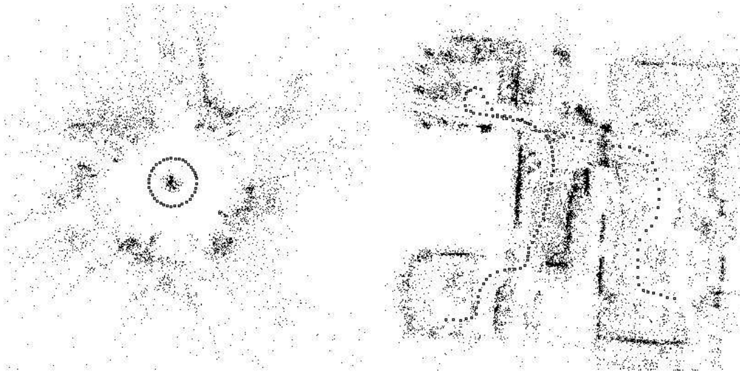
Fig. 7. Top views of Fountain (38 views, 5857 points) and House (112 views, 15504 points) central reconstructions. The Road (54 views, 10178 points) reconstruction is shown in Figure 11. Several of these points are difficult to reconstruct accurately if they are distant or roughly aligned with the cameras from which they are reconstructed. These results are similar for central (with linear and cubic r(\alpha) functions) and non-central models.
