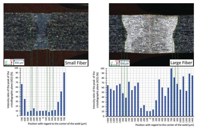
Fig. 8— Location of the X-ray diffraction analysis of Haynes 188 welds obtained in SFC and LFC, respectively (top). Diffraction intensity ratio by the (422) planes of  $M_6C$  precipitates in the weld with respect to the base metal.
