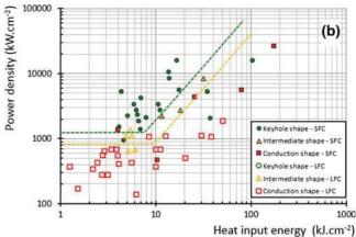
Fig. 1—(a) Domain of weldability of 1.2 mm thick sheets of alloy Haynes 188. (b) Areas of power density and input heat energy values yielding similar weld shapes of Haynes 188.
