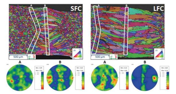
Fig. 6— EBSD inverse pole figure (IPF)  $Z_0$  maps in the LT-ST plane of optimized welds (top). Texture intensity measured in areas A and B (bottom).
