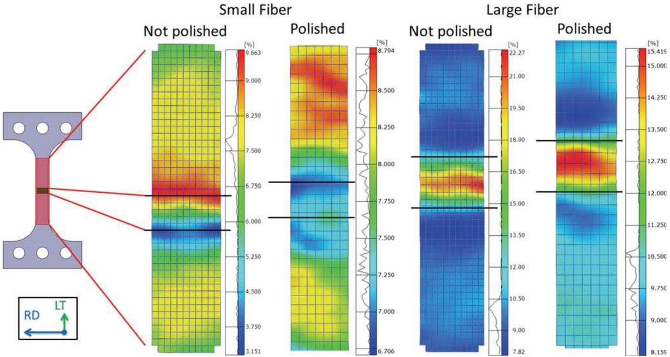
Fig. 10— Comparison of deformation fields in welds at a stress of 750 MPa before and after polishing.
