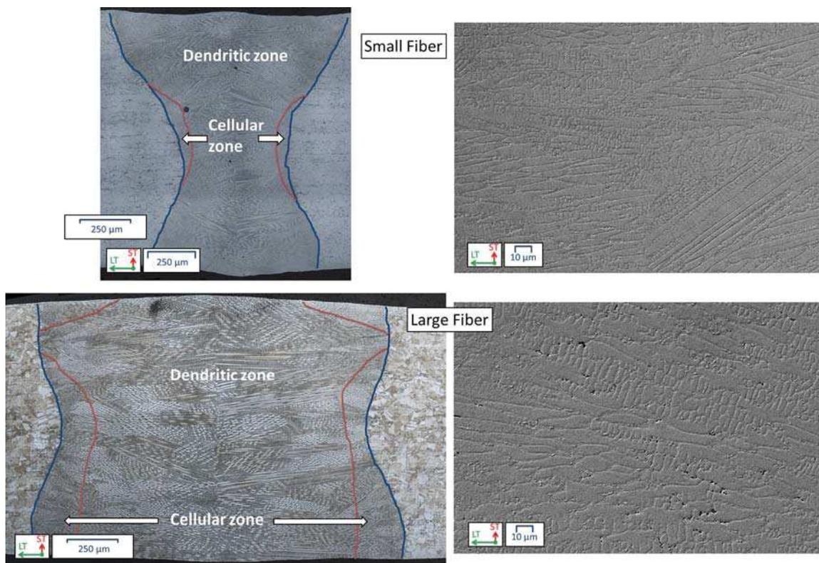
Fig. 4— Dendritic and cellular zones in the welds determined from optical observations at high magnification. SEM micrographs of the center of the welds.
