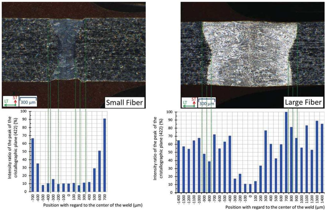
Fig. 8— Location of the X-ray diffraction analysis of Haynes 188 welds obtained in SFC and LFC, respectively (top). Diffraction intensity ratio by the (422) planes of  $M_6C$  precipitates in the weld with respect to the base metal.
