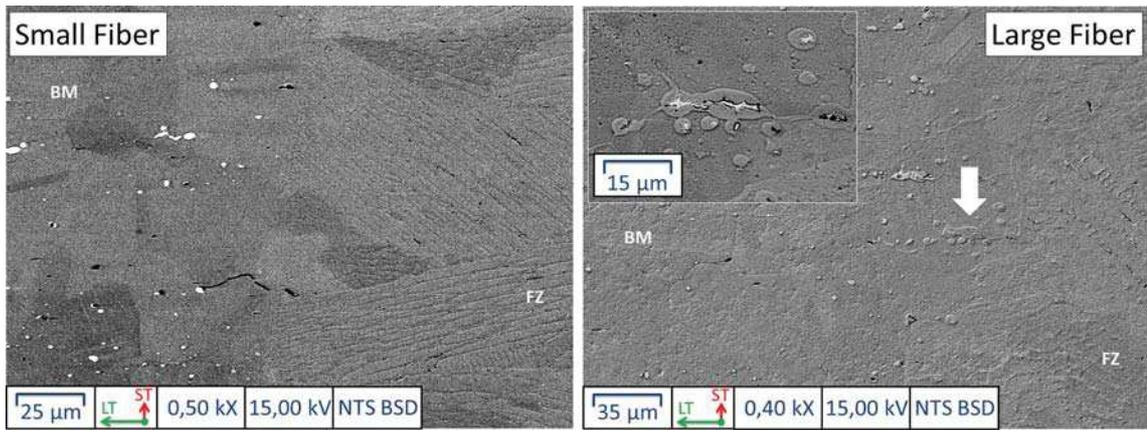
Fig. 3— SEM micrographs (backscattered electron mode) of optimized welds.
