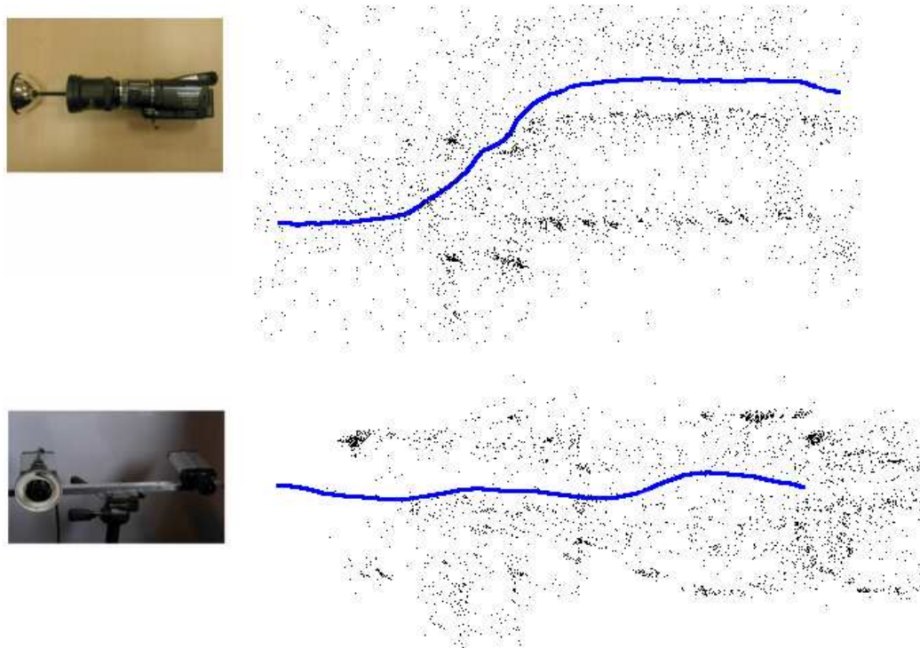
Fig. 18. Cameras and top views of 3D reconstructions. Top: catadioptric camera (Sequence 2). Bottom: stereo rig (Sequence 3). Trajectory in blue and 3D points in black.
