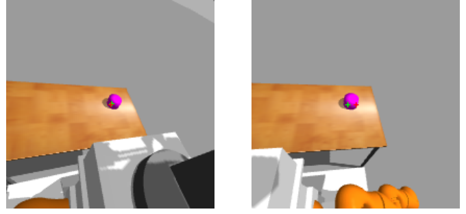
Fig. 1. Binocular fixation achieved on a purple cylinder, the red cross stands for the image center, the green cross is the estimated object pixellic position according to the method described in II-C1b
