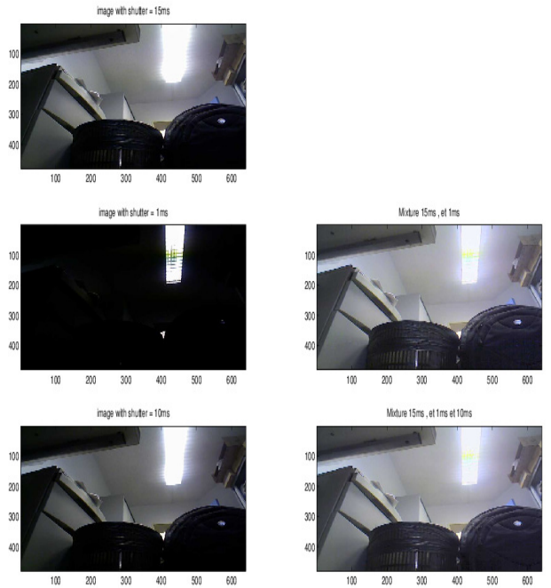
Fig. 9. Static camera : visual improvement of the HDR mixture image obtained from three LDR source images. Since the printer (or screen) dynamic range is not capable of displaying the extended dynamic range the HDR image is remapped to LDR using global tone mapping.
