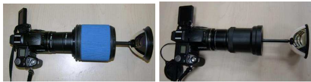
Figure 7: 360 One VR (left) and 0-360 (right) mirrors mounted with the Nikon Coolpix 8700.
