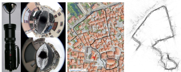
Figure 6. From left to right: our hand-held camera, two images of the sequence, aerial view of the trajectory, the sparse point cloud reconstructed by incremental SfM.
