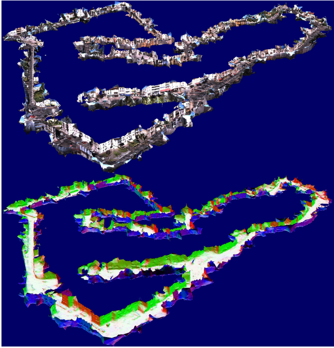
Fig. 8. Global overview of the final surface obtained by our incremental surface reconstruction method including III.B&C as visual artifact removal. We show a textured view (top) and color coded normals (bottom). The triangles on the sky are removed for visualization purposes.
