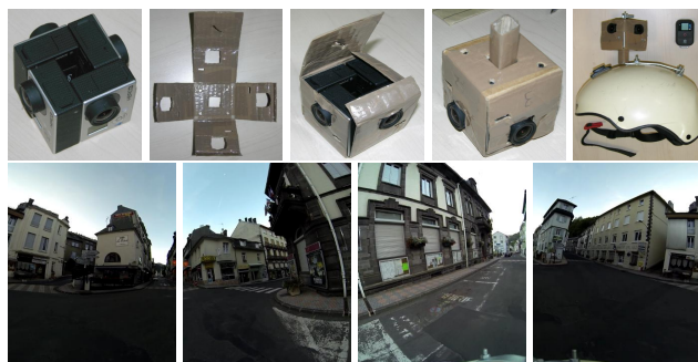
Figure 1. Top: four GoPro Hero3 cameras enclosed in a cardboard box. Bottom: resulting images of our DIY multi-camera.
