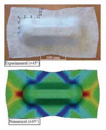
Fig. 14. Experimental and numerical outputs of double dome forming test
