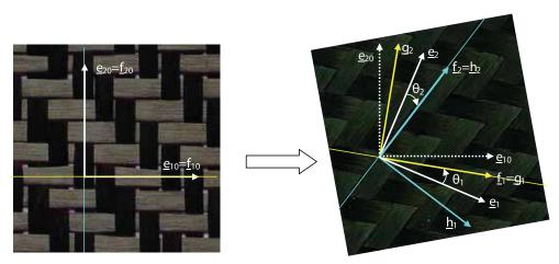
Fig. 11. Fibres axes and GN axes after deformation. Initially these axes are superimposed. The third term  $\overline{W}_s$  in equation (5) is a function of the second mixed invariants of  $\underline{\underline{C}}$ .
