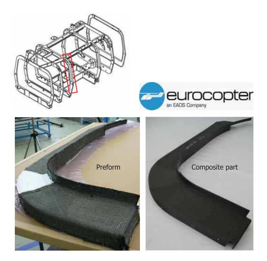
Fig. 1. Preform/RTM parts in NH90 (Dumont et al. 2008) (Courtesy of Eurocopter, EADS Group)
