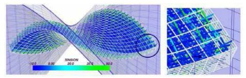
Fig. 24. Forming of a 3D interlock twisted plate
