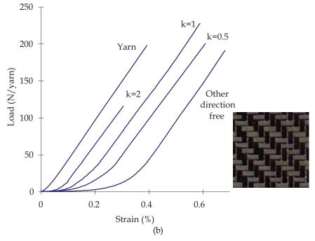
Fig. 6. (a) Biaxial tensile test on cross-shaped specimen (b) Load versus strain for carbon twill weave. k =  $\varepsilon_{warp}$  /  $\varepsilon_{weft}$  (Buet-Gautier et al, 2001)
