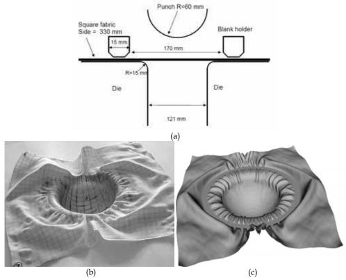
Fig. 21. Forming of an unbalanced textile reinforcement
