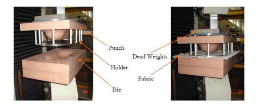
Fig. 13. Double dome forming: experimental device
