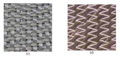
Fig. 4. Textile composite reinforcements (a) plain weave, (b) twill weave (c), interlock, (d) NCF
