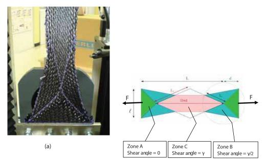
Fig. 8. The bias-extension test and the three zones
