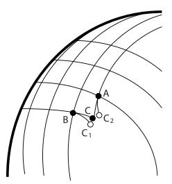
Fig. 3. Fishnet algorithm: Calculation of the position of point C knowing those of A and B
