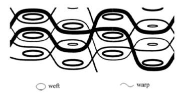
Fig. 22. Example of complex layer interlock weave
