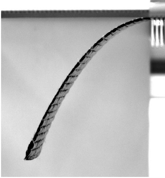
Fig. 10. Cantilever bending test
