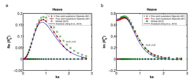
Figure 10: Real and imaginary parts of the Radiation Characteristics progressive terms for a truncated vertical cylinder of 3m radius (a), 6m draft moving in heave in a 10m water depth.
