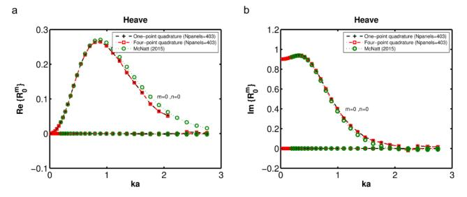
Figure 11: Real and imaginary parts of the Radiation Characteristics progressive terms for a square box of 6m side (2a), 6m draft moving in heave in a 10m water depth.
