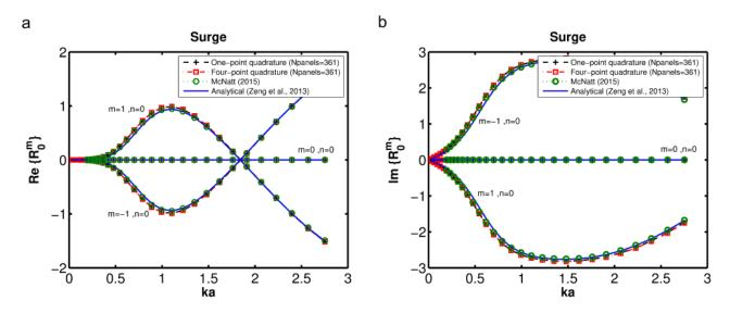
Figure 8: Real and imaginary parts of the Radiation Characteristics progressive terms for a truncated vertical cylinder of 3m radius (a), 6m draft moving in surge in a 10m water depth.
