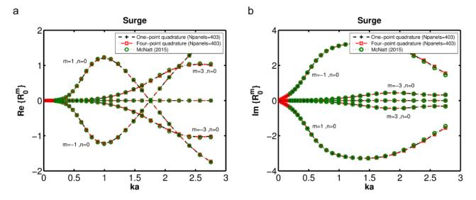
Figure 9: Real and imaginary parts of the Radiation Characteristics progressive terms for a square box of 6m side (2a), 6m draft moving in surge in a 10m water depth.
