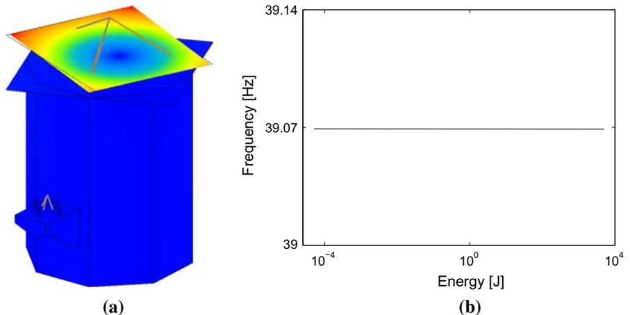
**Fig. 10** FEP of the first NNM with different modal shapes inset
