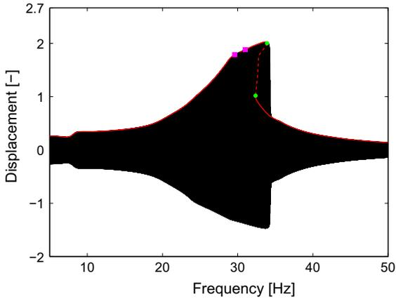
**Fig. 7** SmallSat displacement response at NC2-Z. The responses to swept-sine (direct simulations, 2 octaves per minute) and stepped-sine (numerical continuation) excitations are depicted in *black* and *red*, respectively. The *red solid* and *dashed lines* correspond to stable and unstable periodic solutions, respectively. Limit point and Neimark–Sacker bifurcations are pictured with *green circle* and *magenta squares*, respectively. (Color figure online)
