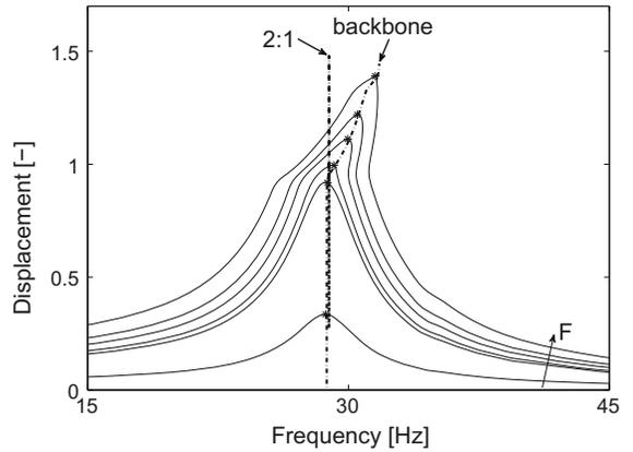
**Fig. 18** Undamped/unforced (*dashed line*) versus damped/forced (*solid line*) response at the WEMS (NC4-Z) in the vicinity of the sixth resonance. Asterisk resonance locus in the damped/forced response
