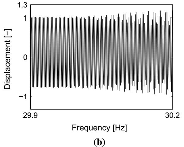
**Fig. 8** Evidence of QP motion. **a** Displacement at NC1-Z and **b** close-up of the transition from periodic to QP motion. The responses to swept-sine (direct simulations) and stepped-sine (numerical continuation) excitations are depicted in *black* and
