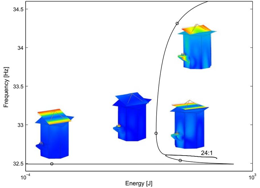
whereas instrument panel motion disappears, giving rise to a localized mode possessing some similarities with LNM6 ( $MAC=0.85$ ). Finally, a motion of the instrument panel, different from the motion at low energy, reappears further on the branch. We note that the localization phenomenon is different from modal interactions. For instance, very little harmonic components are generated along the backbone in Fig. 17.
