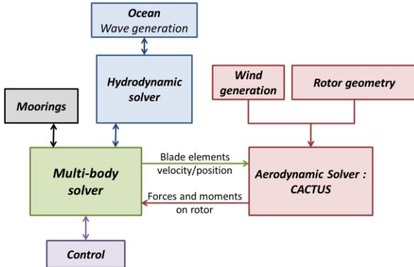
Figure 2: Modular framework coupling InWave and CACTUS
