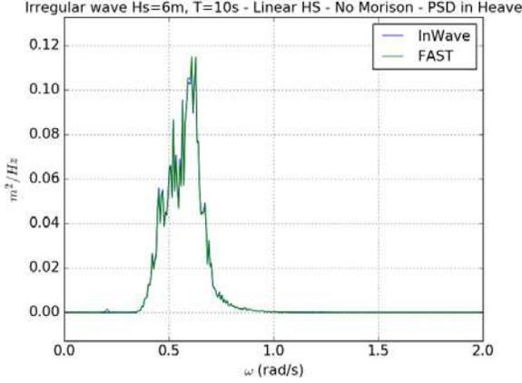
Figure 10: Irregular waves - PSD in Heave
