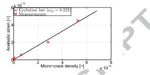
(a) Micro-crack density  $(\gamma_c)$  vs. stress criterion  $(H_c)$  (b) Anelastic strain  $(\varepsilon_{s_{22}})$  vs. micro-crack density  $(\gamma_c)$
