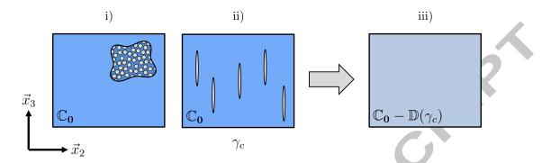
Figure 2: i) Initial state: transversely isotropic. ii) Damaged state: introduction of a micro-cracks density  $\gamma_c$  (void volume fraction) in the RVE. iii) Evaluation of the stiffness reduction induced by  $\gamma_c$  by homogenization.
