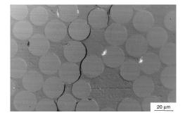
(a) Initiation of the micro-cracks by debonding of the fibre/matrix interfaces
