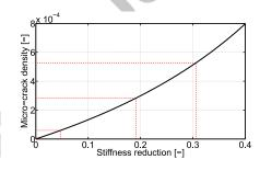
(a) Stress  $(\sigma_{xx})$  vs. strain  $(\varepsilon_{xx})$  curve performed on a  $[90^o]_{16}$  laminate (b) Micro-crack density  $(\gamma_c)$  vs. relative stiffness reduction  $(D_2/E_{02})$
