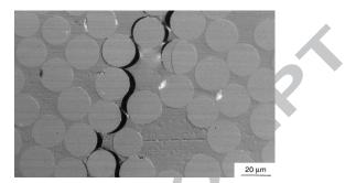
(b) Coalescence into micro-cracks
