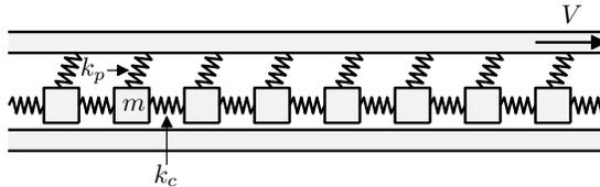
Fig. 1 – Mechanical interpretation of the Burridge-Knopoff model.
