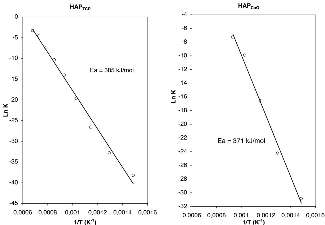
Fig. 10. Activation energy of the sintering phenomenon for HAP<sub>TCP</sub> and HAP<sub>CaO</sub>.
