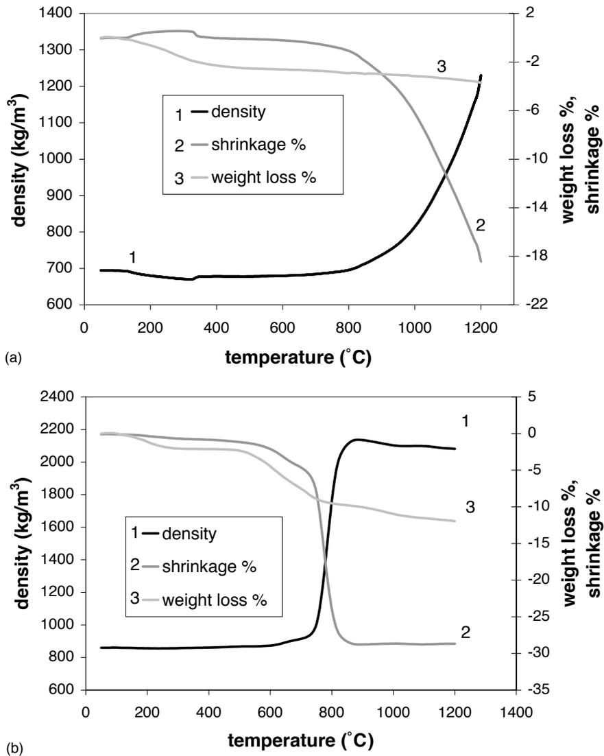
Fig. 8. Shrinkage, density and weight loss (%) of (a) HAP<sub>TCP</sub> and (b) HAP<sub>CaO</sub>.
