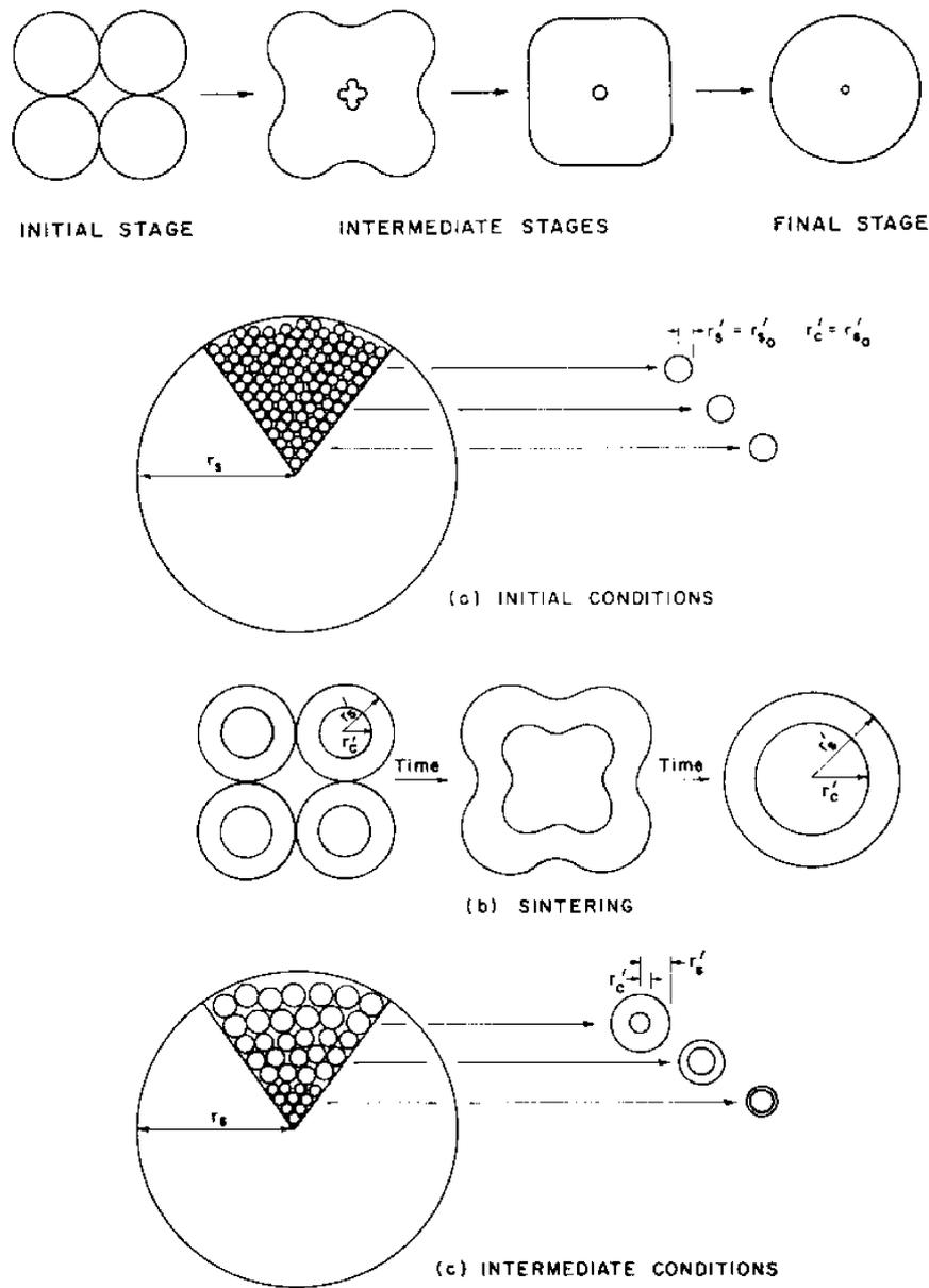
Fig. 1. Sintering phenomenon [13].
