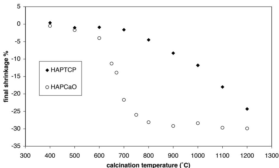
Fig. 6. Final shrinkage (%) vs. the calcination temperature.
