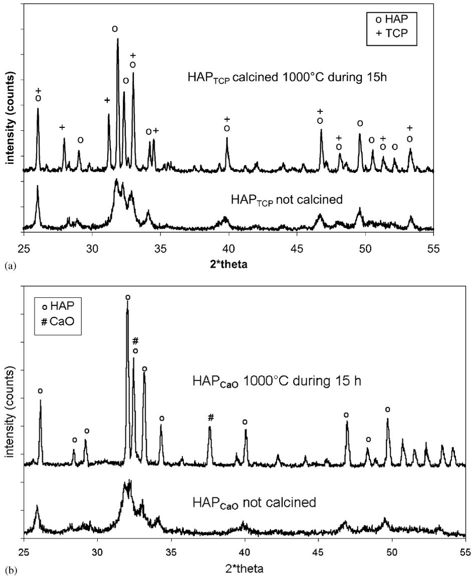
Fig. 4. (a) XRD pattern of (a) HAP<sub>TCP</sub> and (b) HAP<sub>CaO</sub> not calcined and calcined at 1000 °C during 15 h.
