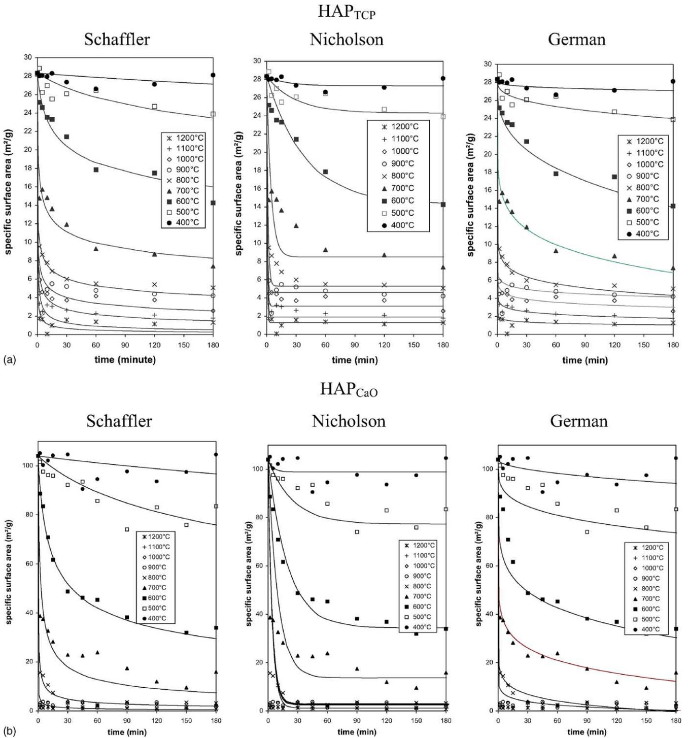
Fig. 9. Modelling of experimental data of surface reduction for (a) HAP<sub>TCP</sub> and (b) HAP<sub>CaO</sub>.
