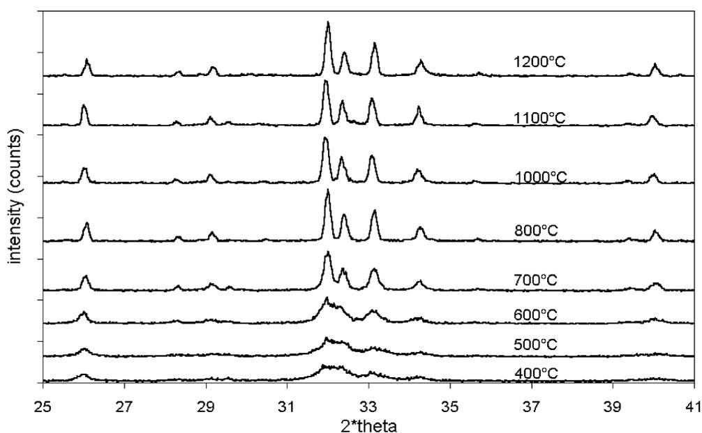
Fig. 3. XRD pattern of HAP<sub>CaO</sub> vs. the calcination temperature.
