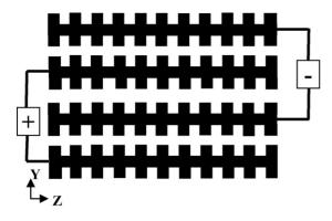
Fig. 5. Experimental electrode geometry: periodic, aligned, castellated bars of electrodes, represented by the blackened areas. The electrode width and spacing between the electrodes are both  $100 \,\mu$ m.
