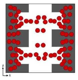
Fig. 4. Positions of the particles at time t = 1.0 s from the numerical simulation, showing streaks of particles aligned in the *z*-direction on top of the electrodes and bridges in the wells in between the electrodes.
