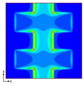
Fig. 2. Electric field distribution in the plane of the electrodes from the numerical simulation.
