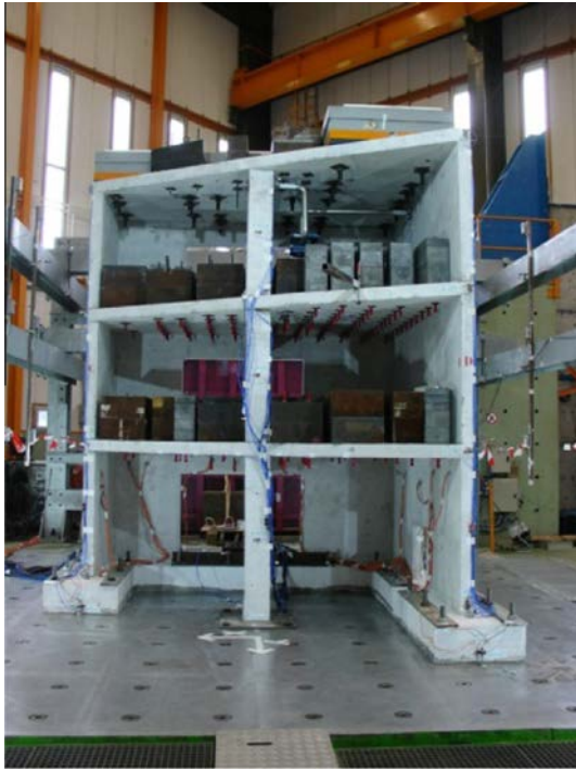
Fig. 2. Picture of the SMART 2013 fixed on the AZALEE shaking table ready to be tested.
