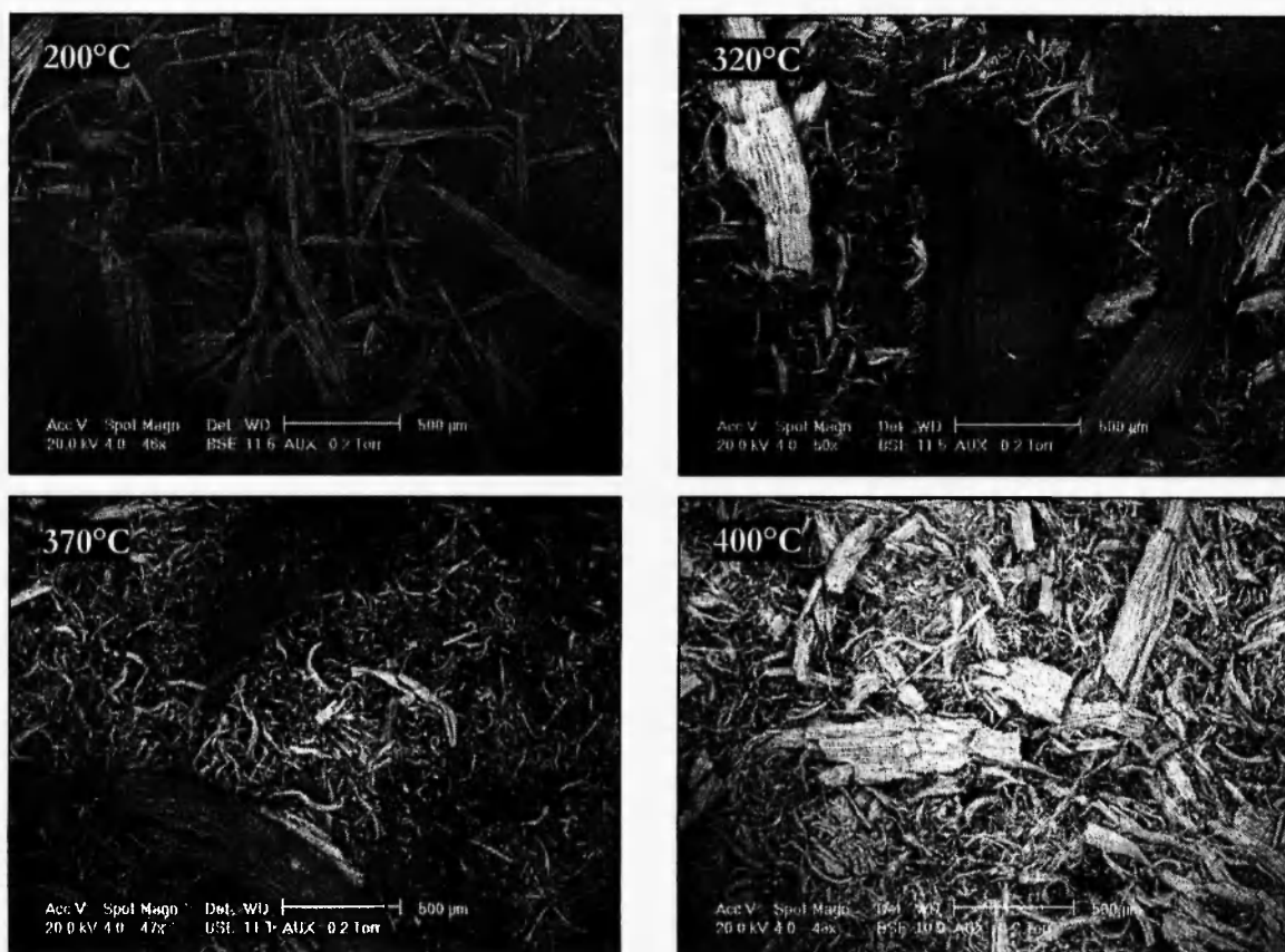
Fig. 3: Environmental scanning electronic micrographs (ESEM) of CCA treated wood residues at different pyrolysis temperatures (heating rate=20°C/min and pyrolysis duration= 90min).
