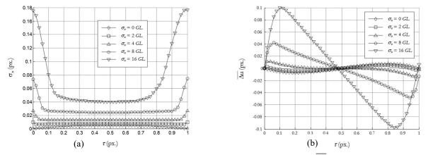
Figure 1.a – Evolution of the random error  $\sigma_u$  and 1.b – evolution of the bias error  $\Delta u$  as a function of imposed displacement  $\tau$  for different noise levels  $\sigma_n$  for d = 16 px.
