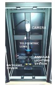
Fig. 6. Photograph of the detection prototype
