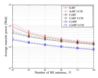
Fig. 6. Average transmit power in Watt vs. N when L = 16, K = 8 and the rates are randomly taken in the interval [1, 3].
