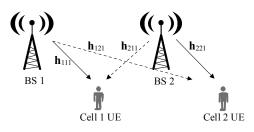
Fig. 1. Graphical representation of a simple two-cell network with one UE per cell such that  $d_{111} = d_{211} = d_{221} = d$  and  $d_{121} = \alpha d$  with  $\alpha < 1$ .
