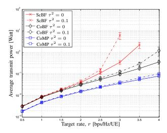
Fig. 3. Average transmit power in Watt vs. target rate when L = 16, K = 8 and N = 32.
