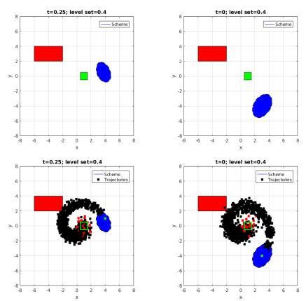
FIGURE 3. (Example 1). Top: backward reachable set (blue region) at times  $t \in \{0.25, 0\}$  for a final time horizon T = 1.75 in presence of the obstacle (red rectangle). Bottom: reconstruction of some optimal paths starting from point  $\bar{x} = (4, 1)$  (bottom, left) and  $\bar{x} = (3, -4)$  (bottom, right).
