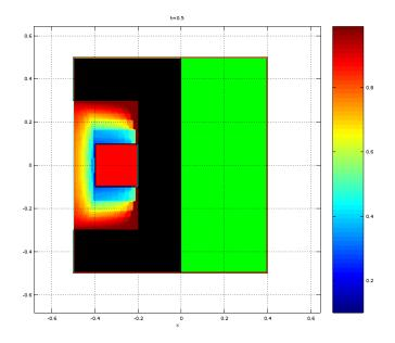
FIGURE 4. (Example 2) approximation of  $\Omega_t^{\rho}$  at t = 0 for different levels  $\rho \in [0, 1, 0.9]$  computed with  $\Delta x_1 = \Delta x_2 = 0.005, \Delta y = 0.1, h = 0.01$  (same mesh parameters used in [10]).
