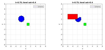
FIGURE 2. (Example 1) Backward reachable sets at t = 0.75 for a time horizon T = 1.75 and  $\rho = 0.4$  without (left) and with (right) obstacle. The target set, the obstacle and the backward reachable set  $\Omega_{0.75}^{0.4}$  are represented respectively by the green square, the red rectangle and the blue region.
