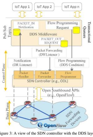
Figure 3: A view of the SDN controller with the DDS layer
