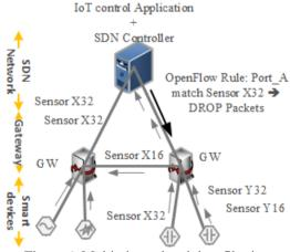
Figure 6: Multi-channel and data filtering
