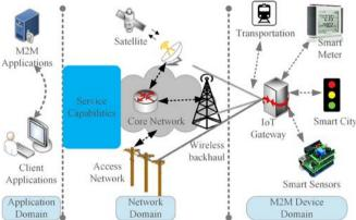
Figure 2: High-level IoT architecture
