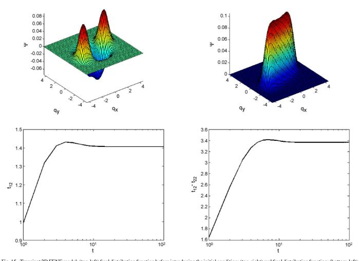
Fig. 15. Transient 2D FENE model: (top-left) final distribution function before introducing the initial condition; (top-right) real final distribution function; (bottom-left) shear stress evolution and (bottom-right) evolution of the first normal stress difference.
