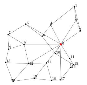
FIG. 1. Optimal solution of a HSNDP instance with K = 3 and H = 3; n = 21,  $D = \{(0, v) : v = 1, ..., 20\}$ , complete graph, Euclidean costs.
