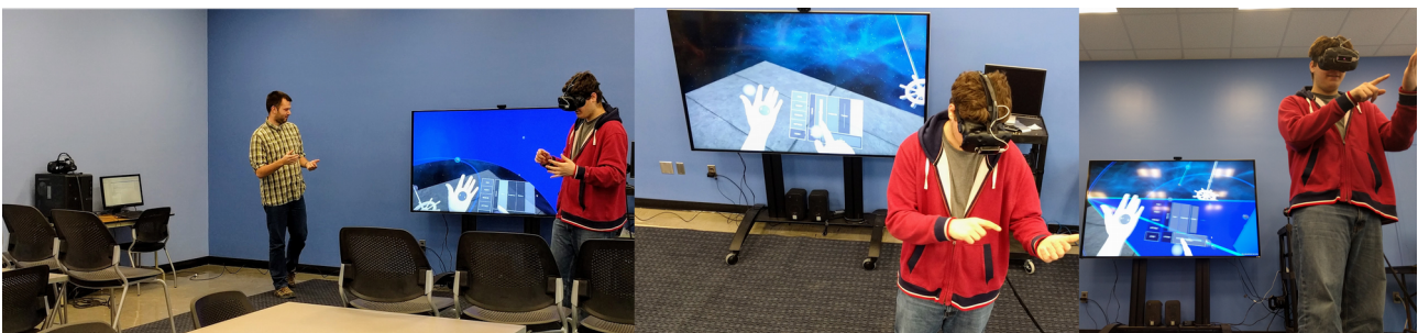
Figure 2. A user (red sweatshirt) in the virtual space. The large monitor displays a 2D view of the user's first-person view of the virtual world. The device that tracks the user's hand movements is mounted to the front of the headset he is wearing.
