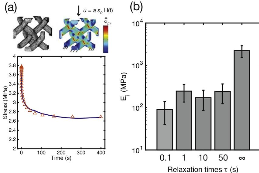
**Fig. 8.** Time domain simulations FEM. (a) Time domain simulation of BD structures. The solid line represents the experimental data and the triangular markers the simulation results. The insets show the FEM mesh (left) and the von Mises stress distribution (right). (b) Calculation of the individual branch moduli for the generalized Maxwell model, as a function of different relaxation times. The error bars stem from the variance of experiments using all samples as reported in Table I.
