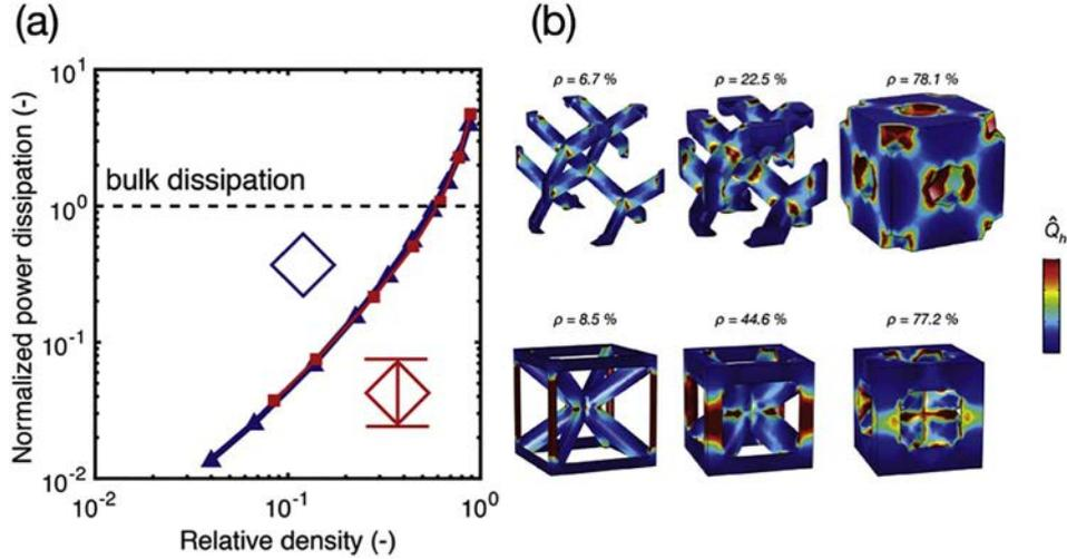
**Fig. 9.** Frequency domain simulation. (a) Power dissipation per cycle as a function of relative density for the two lattice geometries considered: BD (blue) and SD (red). (b) Von Mises stress distribution for varying densities of BD (top row), SD (bottom row) structures. (For interpretation of the references to color in this figure legend, the reader is referred to the web version of this article.)
