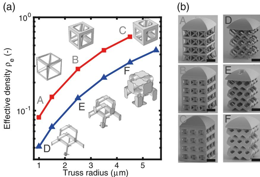
**Fig. 2.** Varying unit cell densities. (a) Effective lattice densities as a function of truss radius  $r$  for SD (red) and BD (blue) structures. (b) Panels A-F showing SEM micrographs of fabricated micro-compression samples with varying truss radius, scale bar is  $25\ \mu\text{m}$ . (For interpretation of the references to color in this figure legend, the reader is referred to the web version of this article.)
