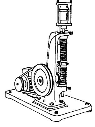
Fig. 1. One-ball vibration mill of type Dangoumau.
