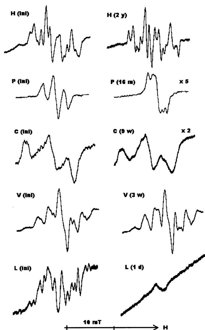
Fig. 3. EPR spectra of some irradiated amino-acids (H = histidine, P = proline, C = cysteine, V = valine, L = leucine; ini = just after irradiation, y = year, m = month, w = week, d = day; other recording conditions in the text).
