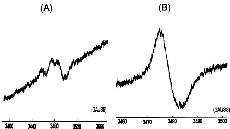
Fig. 5. EPR spectra of radicals induced by grinding in lactose (A) and carboxymethylcellulose (B).
