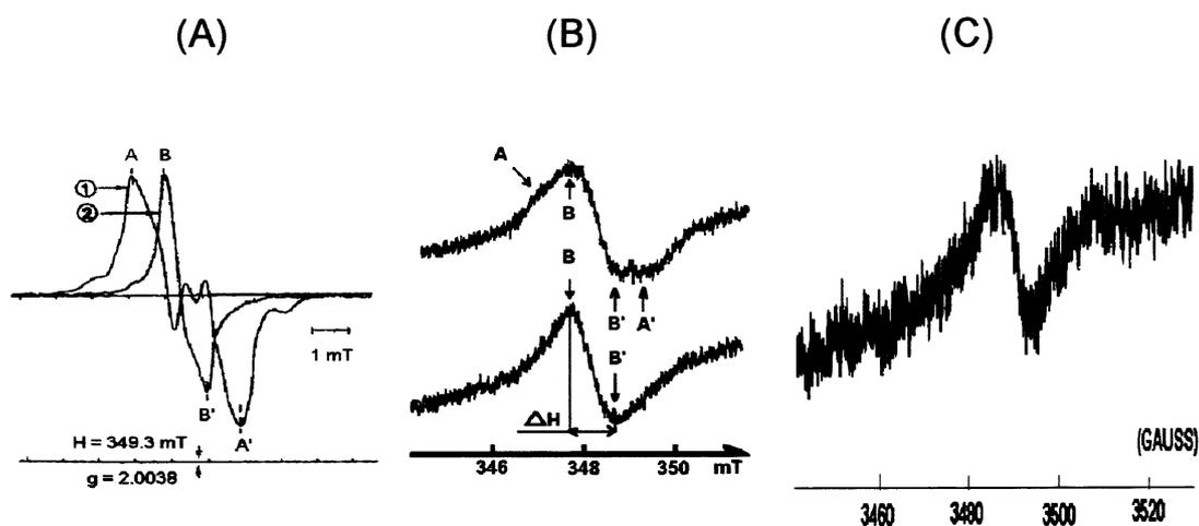
Fig. 4. EPR signals of radicals induced in starches by gamma radiation (A), UV radiation (B) or grinding (C). (A) Curve 1 recorded just after gamma irradiation, curve 2 recorded 6 months later (gain multiplied by 20). (B) Upper curve recorded just after UV irradiation, curve 2 recorded several hours later.
