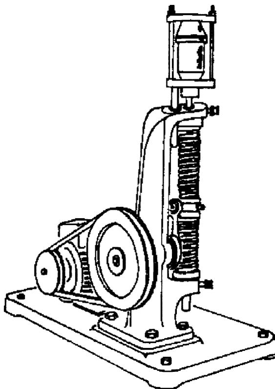
Fig. 1. One-ball vibration mill of type *Dangoumau*.
