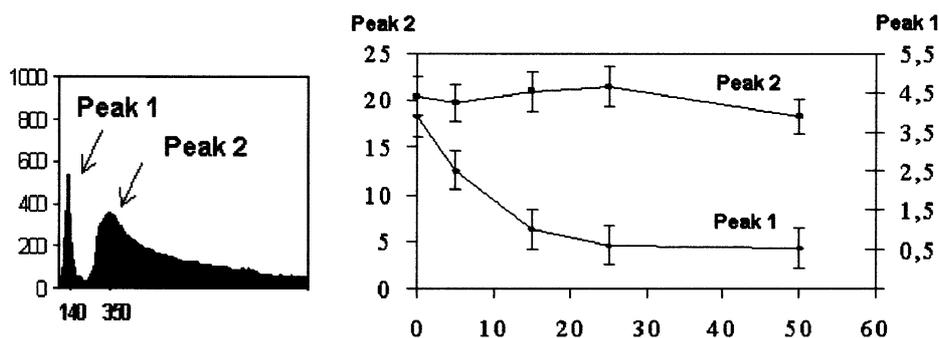
Fig. 6. TL recording (left) of unirradiated anhydrous ampicilline acid and variation of peak intensities (right) with irradiation dose (kGy).
