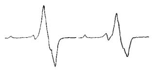
Fig. 2. ESR spectra of radicals induced in anhydrous ampicilline acid just after a 50 kGy irradiation (left) and six months later (right).
