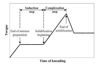
Fig. 11. Scheme of successive main steps occurring during kneading process.
