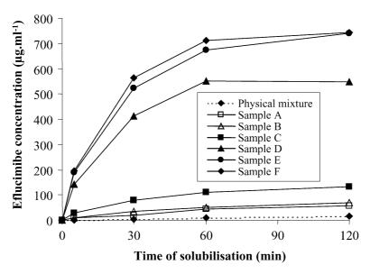
Fig. 8. Evolution of eflucimibe solubilisation kinetics during kneading process.
