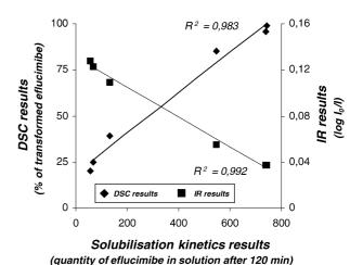
Fig. 9. Representation of DSC results and IR results in relation to solubilisation kinetics results.
