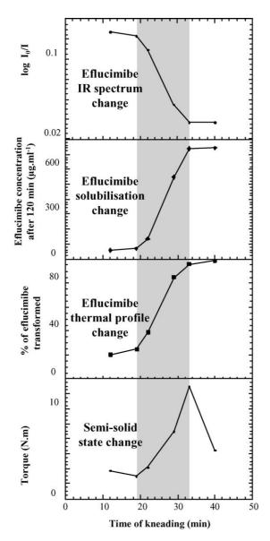
Fig. 10. Representation of the evolution of physico-chemical and semi-solid states of the eflucimibe:  $\gamma$ -cyclodextrin mixture during kneading process.
