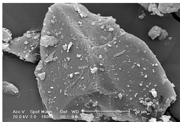
Fig. 7: Surface morphology of particles coated with 1% magnesium stearate using the Hybridizer.
