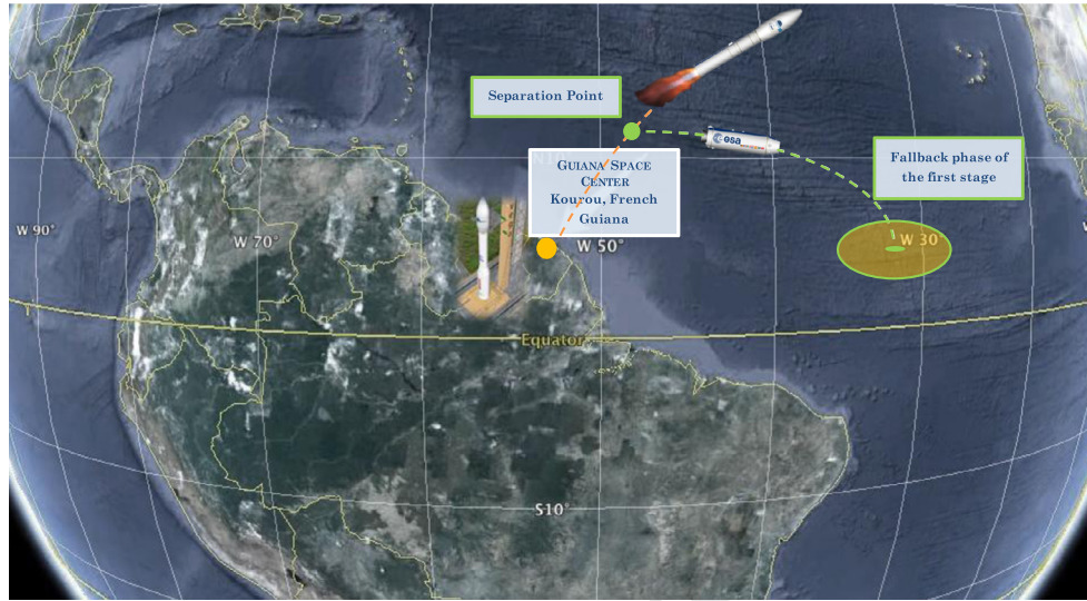
Fig. 3. Illustration scheme of the first stage fallback phase into the Atlantic Ocean.
