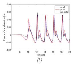
Figure 12: Comparisons between the experimental data (solid line) and the simulations of the dispersive model with  $\gamma = \sqrt{3}$  (blue dashed line) and  $\gamma = \sqrt{5}$  (red dashed-dotted line). Figs. (a), (b) respectively correspond to the results for the sensors 4 and 5.
