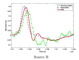
Figure 17: Comparison between numerical results using both models (hydrostatic and non-hydrostatic) and the data of the DART buoy 32401 for (a) source A and (b) source B.
