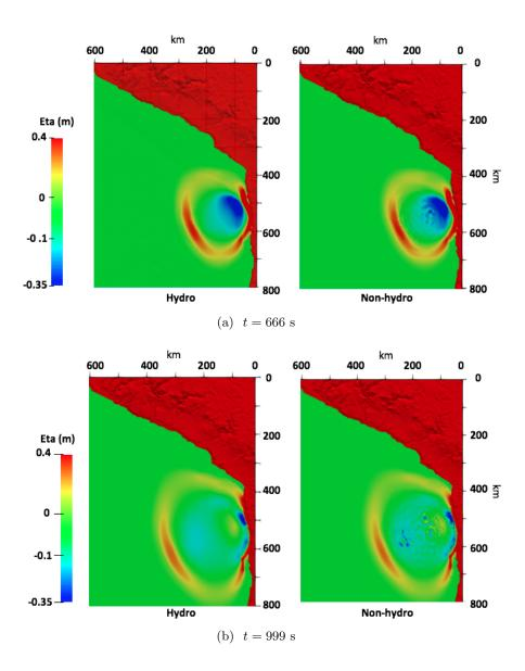
Figure 16: Comparison of the wave front for the hydrostatic (left) and the non-hydrostatic (right) model at time t = 666s and t = 999 s and using the source A. The coordinate (0,0) corresponds to the coordinate (15.0 S, 70.0 W).
