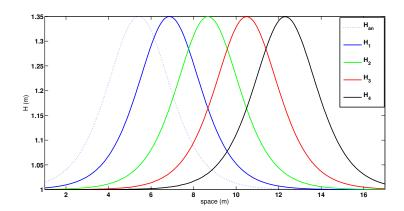
Figure 6: Cross section at the center of the channel y = 0.5 m; water depth of the analytical solution at initial time  $H_0 = H_{an}$  and computed solution  $H(t_i)$ , i = 1, ..., 4 with  $t_0 = 0$  s,  $t_1 = 0.499805$  s,  $t_2 = 0.999871$  s,  $t_3 = 1.49983$  s,  $t_4 = 1.99993$  s for the P<sub>1</sub>-isoP<sub>2</sub>/P<sub>1</sub> approximation and the improved method (Heun scheme).
