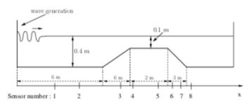
Figure 10: Channel profile for the experiments and location of the sensors.
