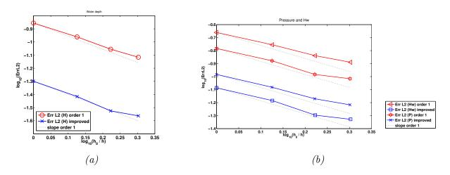
Figure 9: Convergence rate: (a) of the  $L^2$  error of the water depth and (b) of the vertical discharge and the pressure.
