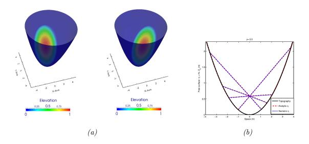
Figure 8: (a) Simulation of the free surface oscillations in a paraboloid at different time steps and (b) cross section of the free surface at y=0 of the free surface  $H+z_b$  compared with the analytical solution at different times:  $t_0=0.277222$  s,  $t_1=0.431123$  s,  $t_2=0.739382$  s,  $t_3=0.893419$  s ans  $t_4=1.20134$  s.
