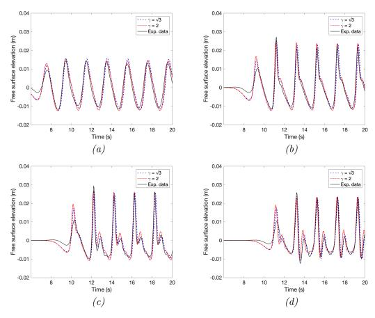
Figure 11: Comparisons between the experimental data (solid line) and the simulations of the dispersive model with  $\gamma = \sqrt{3}$  (blue dashed line) and  $\gamma = 3/2$  (red dashed-dotted line). Figs. (a), (b), (c) and (d) respectively correspond to the results for the sensors 3, 4, 5 and 6.
