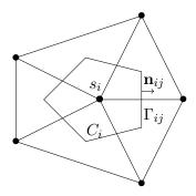
Figure 2: Representation of the dual mesh
