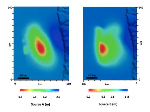
Figure 14: Imposed displacement for (a) source A and (b) source B. The selected zone corresponds to the source zone in red shown in Fig. 13.
