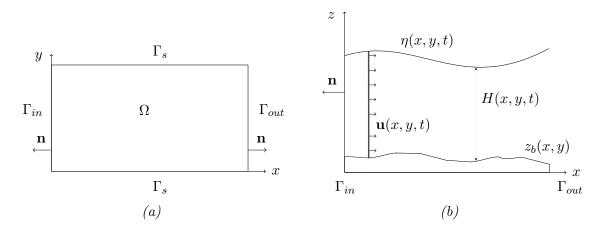
Figure 1: Model domain and notations, (a) view from above and (b) vertical cross section.
