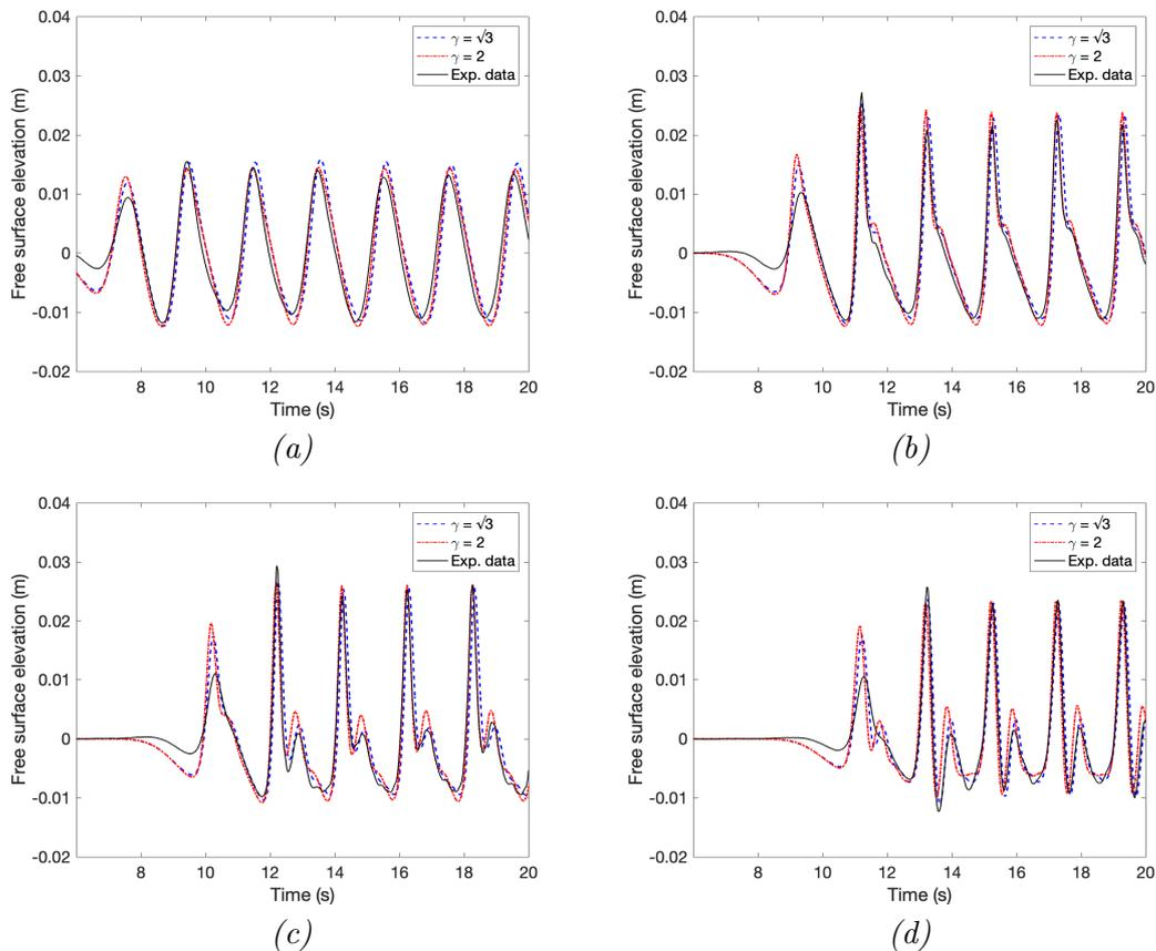
Figure 11: Comparisons between the experimental data (solid line) and the simulations of the dispersive model with  $\gamma = \sqrt{3}$  (blue dashed line) and  $\gamma = 3/2$  (red dashed-dotted line). Figs. (a), (b), (c) and (d) respectively correspond to the results for the sensors 3, 4, 5 and 6.
