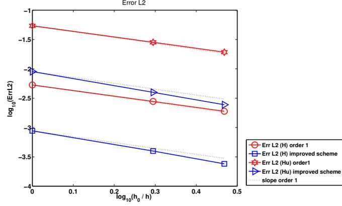
Figure 7: Convergence rate for the  $P_1$ -iso $P_2/P_1$  approximation for the classical scheme (order 1 in time and space) and the improved method (Heun scheme and reconstruction in the prediction step). The  $L^2$  error is computed at time  $t = 1.99s$
