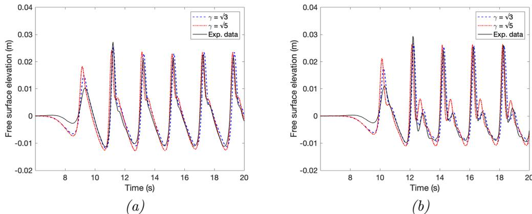
Figure 12: Comparisons between the experimental data (solid line) and the simulations of the dispersive model with  $\gamma = \sqrt{3}$  (blue dashed line) and  $\gamma = \sqrt{5}$  (red dashed-dotted line). Figs. (a), (b) respectively correspond to the results for the sensors 4 and 5.
