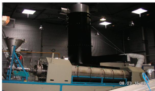
Figure 1. The pilot rotary kiln.
