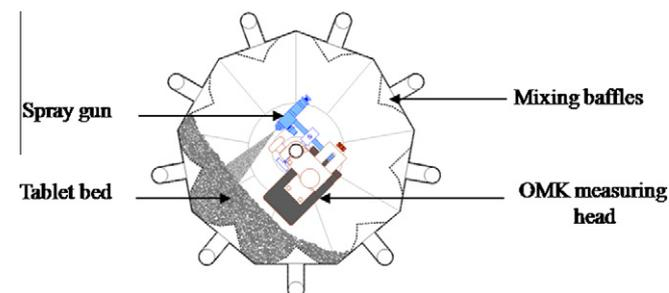
Fig. 1. Schematic integration of the probe inside the pan coater.
