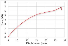
Fig 10: Force-Displacement behavior for OSB panel.
