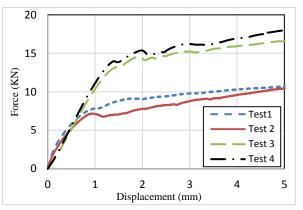
Fig 4: wood compressive strength transverse to the grain.
