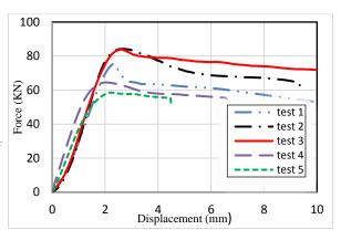
Fig 3: wood compressive strength Parallel to the grain
