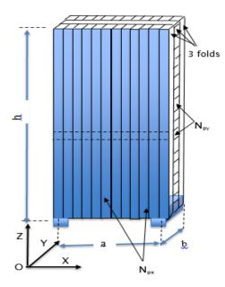
Fig 1: The formation of the cross plank wall unit.
