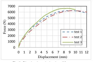
Fig 5: Simple shear behavior of fasteners.
