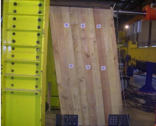
Fig 7: Timber cross plank wall in test.
