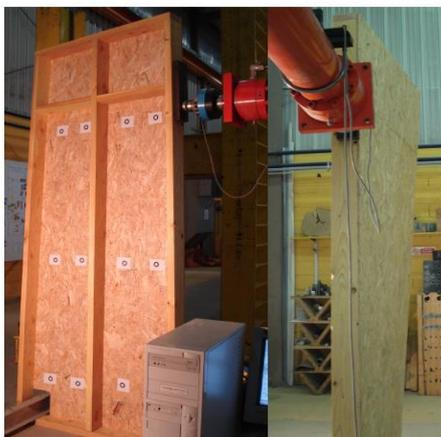
Fig 9: OSB panel in test.
