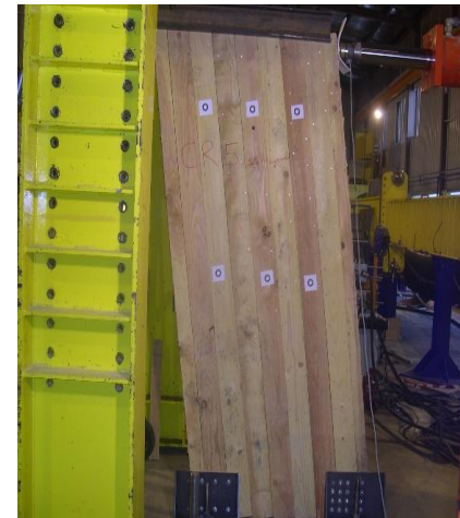
Figure 4: Timber cross plank wall in test.
