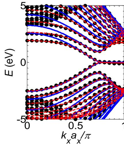
FIG. 6. Comparison of energy bands for a zigzag graphene ribbons of width  $M = 11$  with DFT (black with filled circle), the 3NN TB model using the set of Gunlycke (blue) and the 3NN TB model using the set proposed in this work (red).
