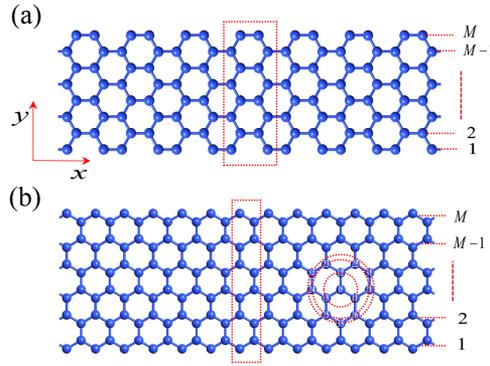
FIG. 1. Two typical ribbon structures with (a) armchair edges and (b) zigzag edges. The width of the ribbons is characterized by the parameter  $M$  referring to the number of dimer lines in armchair ribbons and to the number of chain lines in zigzag ribbons.
