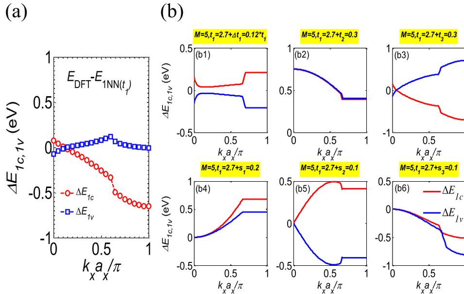
FIG. 3. (a) Difference of energy in the first conduction ( $\Delta E_{1c}$ ) and the first valence ( $\Delta E_{1v}$ ) bands between DFT and simple 1NN TB calculations. (b) The quantities  $\Delta E_{1c}$  and  $\Delta E_{1v}$  were calculated to show the impact of each single TB parameter, as the difference between results of [1NN + 1 parameter] and 1NN TB calculations. All calculations were performed for the armchair ribbon of width  $M = 5$ .
