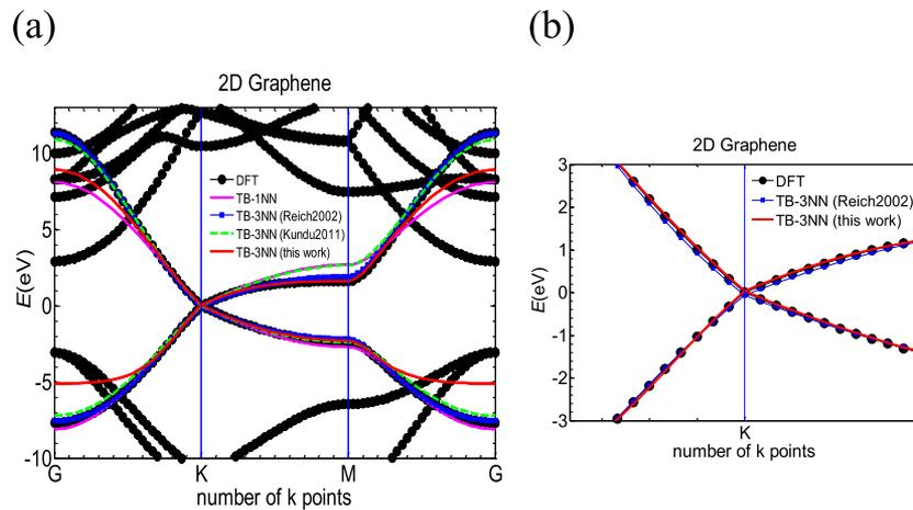
FIG. 7. (a) The band structure of 2D graphene sheet: Comparison between the DFT data and the ones obtained by different TB models. (b) Zoom in on the low energy region around the Dirac point (K point).
