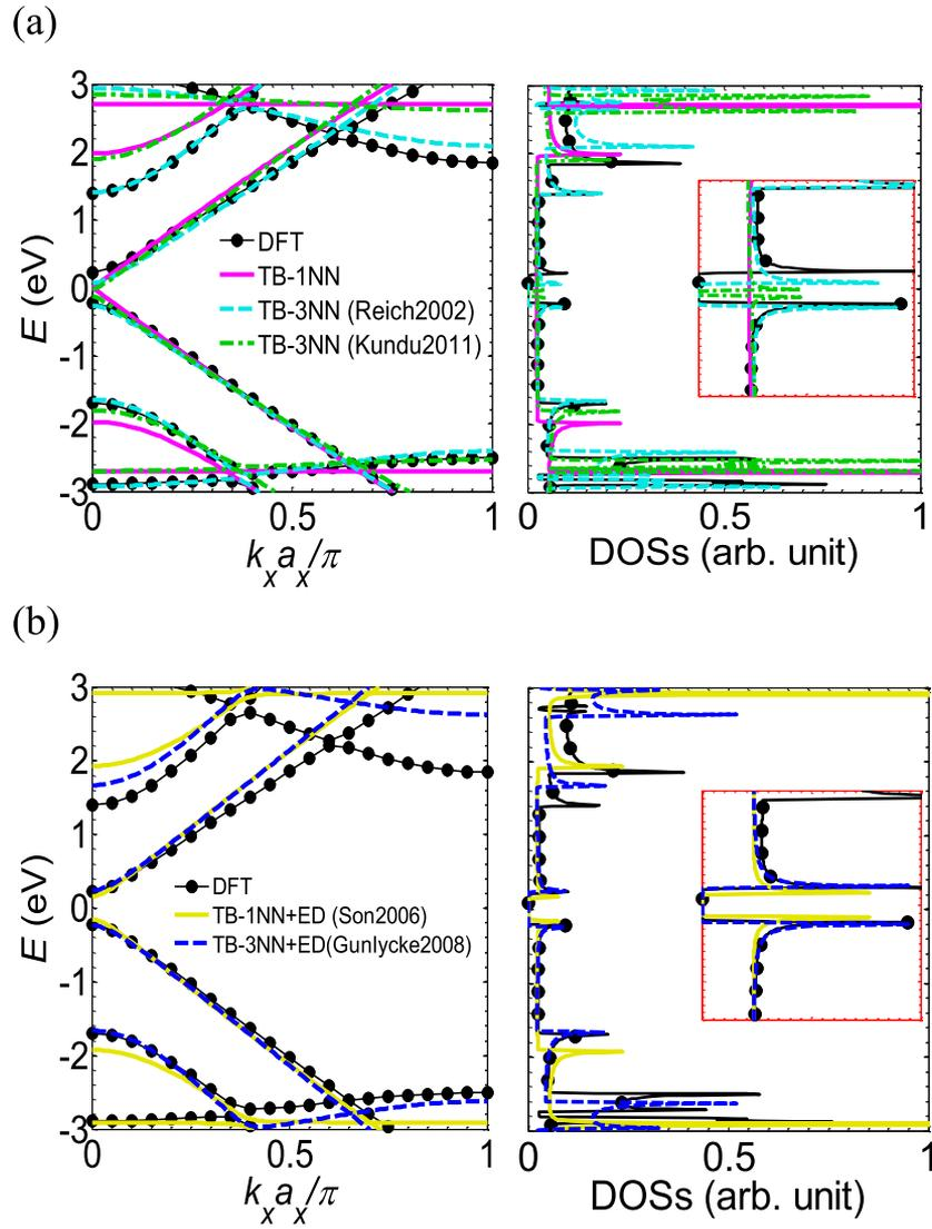
FIG. 2. Comparison of energy bands and density of states (DOSs) for an armchair ribbon of width  $M = 5$  calculated by DFT and TB method. (a) Using sets of TB parameters fitted for 2D graphene. (b) Using sets of TB parameters fitted for graphene ribbons.
