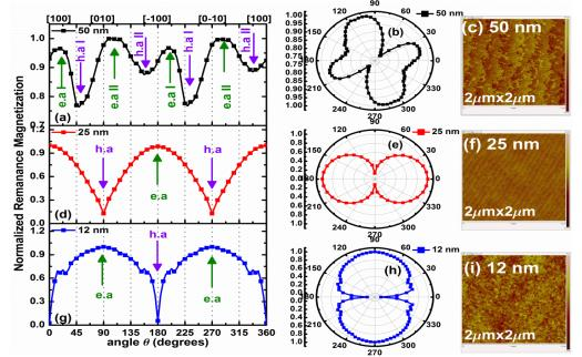
Figure 1: (a, d and g) v-MOKE angular dependent remanence magnetization of LSMO films of varying thickness grown on STO (001) substrate; (b, e, h and c, f, i) are the corresponding polar plots and AFM topography respectively.
