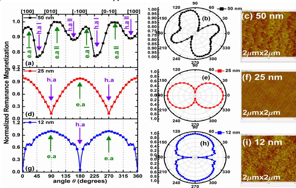
**Figure 1:** (a, d and g) v-MOKE angular dependent remanence magnetization of LSMO films of varying thickness grown on STO (001) substrate; (b, e, h and c, f, i) are the corresponding polar plots and AFM topography respectively.
