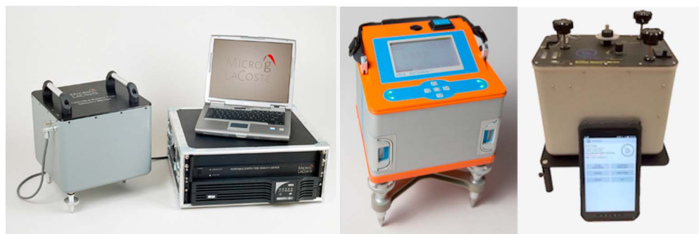
Figure 5. Three relative gravimeters: (left) Micro-g LaCoste gPhone (metal spring); (middle) Scintrex CG-6 Autograv (quartz spring); (right) Burris gravimeter (metal spring). Credit: Micro-g LaCoste, Scintrex Ltd, and ZLS Corporation.
