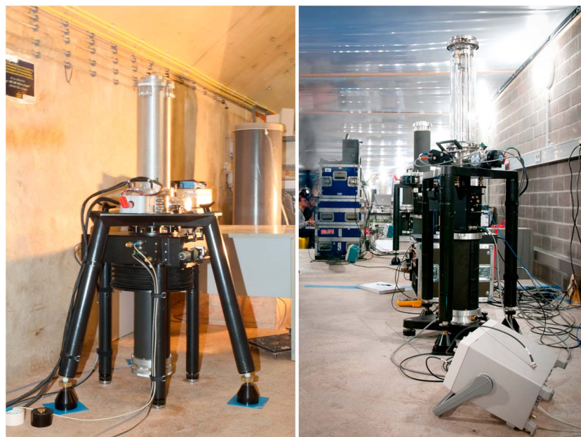
Figure 2. (left) The FG5#202 absolute gravimeter at the Membach station, Belgium and (right) an FG5X at the Walferdange station, Luxembourg. The box with the red connector is the ion pump, maintaining a vacuum in the dropping chamber (upper cylinder) at the 10^{-9} atmosphere level. Credit: K. Vanneste, Royal Observatory of Belgium (Figure 2, left), O. Francis, U. Luxembourg (Figure 2, right).
