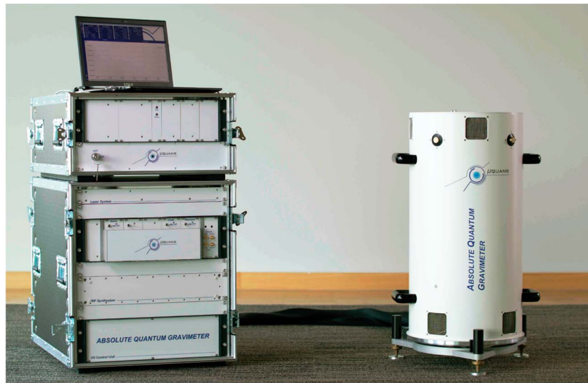
Figure 3. The Muquans absolute quantum gravimeter, based on laser-cooled atoms. Credit: Muquans.
