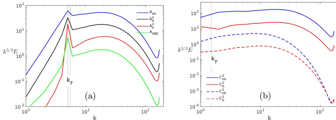
**Figure 3.** Spherically integrated kinetic energy spectra: (a) for runs in set A ( $k_F \simeq 5$ ); (b) for runs in set C ( $k_F = 1.5$ ). Spectra are shifted vertically for better view, and are compensated by the Kolmogorov inertial scaling  $k^{5/3}$ .  $k_F$  indicates the forcing wavenumber, as in the following plots.
