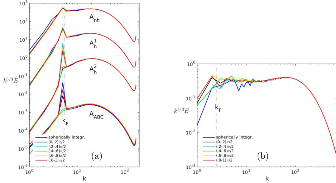
**Figure 4.** Directional energy spectra  $E_i(k)$  compensated by  $k^5/3$ , as functions of wavenumber  $k$  for the five angular sectors for: (a) set A ( $k_F = 5, 5.5$ ); (b) run  $D_{nv}$ . The five sectors are indicated in legend, and the same colorcode applies throughout the paper.
