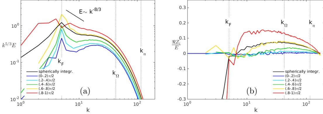
**Figure 17.** Helical shell-Euler forced run: the truncated system includes wavenumbers such that  $4.6 \leq k \leq 5.4$  and does not include the Coriolis force. The parameters of the simulation are  $Re^\lambda = 180$ ,  $Ro^\omega = 1.13$ ,  $H_{rel} = 0.50$ . (a) Directional energy spectra; (b) real part of polarization normalised by the energy spectrum.
