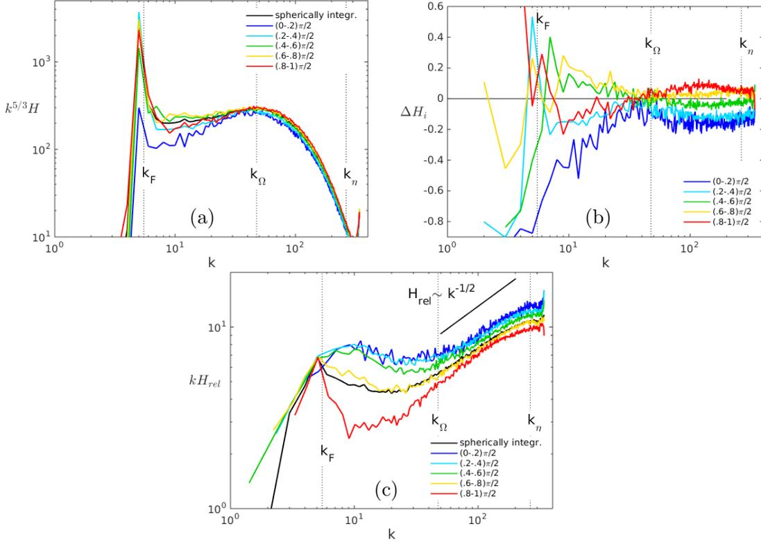
**Figure 20.** (a) Directional helicity spectra  $H(k, \theta)$  compensated by  $k^{5/3}$ , (b) helicity directional anisotropy  $\Delta H_i(k)$ , (c) relative helicity directional spectra  $H_{rel_i}(k) = H_i(k) / (2kE_i(k))$ , for run  $S_h$ .
