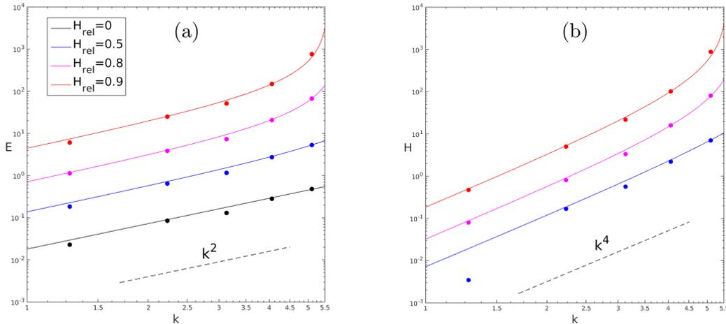
**Figure 2.** Exact energy and helicity spectra of the spherically truncated Euler system for different relative helicities (continuous line) and DNS time-averaged spectra (markers). The truncation wavenumber is  $k_F = 5.5$ .
